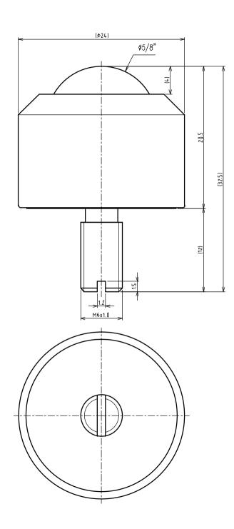
>Description IS-N Type Ball Transfer With Sturdy Bolt IS-16N Type Unit = mm
