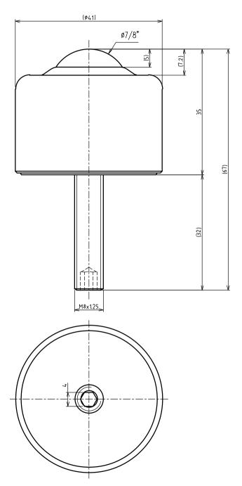
>Description IS-SN Type Ball Transfer With Sturdy Bolt IS-19SN Type Unit = mm
