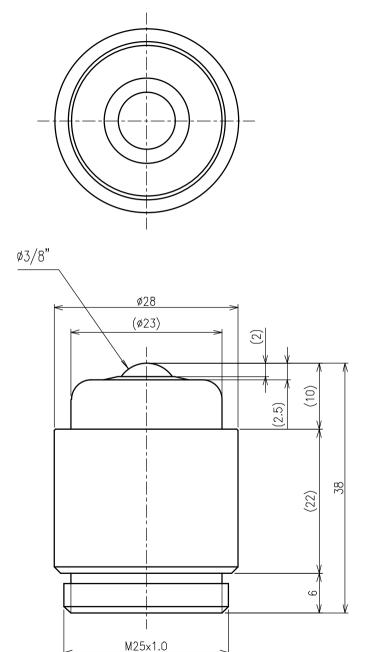
>Description IS-B Type Spring Ball Transfer IS-10B Type Unit = mm
