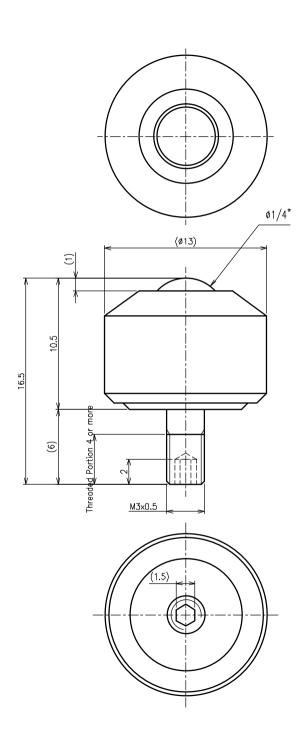
>Description IS—SNM Type Ball Transfer With Sturdy Bolt IS—06SNM Type Unit = mm
