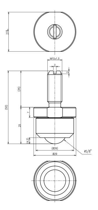
>Description IK-SNM Type Ball Transfer With Sturdy Bolt IK-16SNM Type Unit = mm
