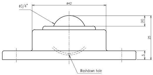
>Description IJP Type Ball Transfer IJP-19 Type Unit = mm
