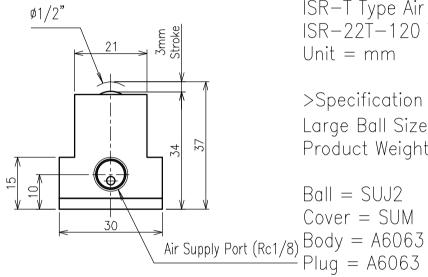
>Description ISR-T Type Air Ball Lifter ISR-22T-120 Type Unit = mm
